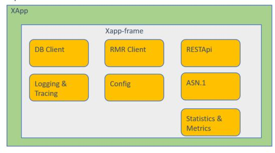
The common functions and interfaces that the xApp-framework provides include:
