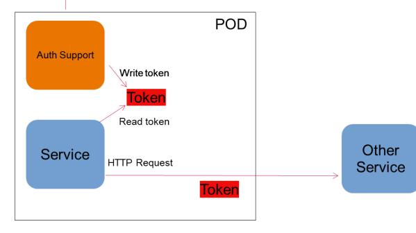
How an rApp's μService uses authorisation tokens – automatically enabled at instantiation time ... a few different options
