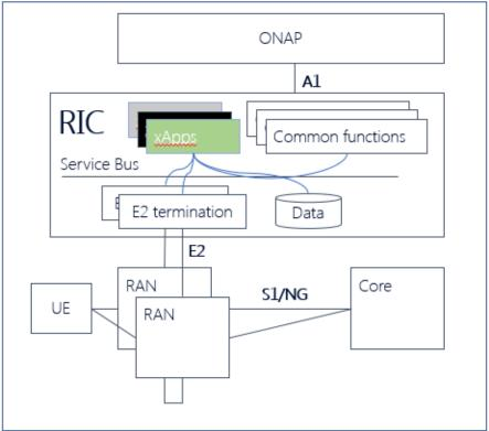
RIC platform contains E2 termination, shared data and common functions to form the "RIC Platform", running on a PaaS platform.
