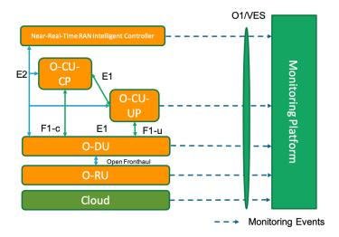
Another view of the same can be seen in the diagram below. In this case the events are picked up by the VES Agents which formats them in the form of a VES Event and sends it towards the VES Collector. The VES Collector stores the events in InfluxdB and alternatively to the Elasticsearch engine and/or the Kafka bus. The event data can then be picked up by Grafana or any other application to perform any analysis on the data.
