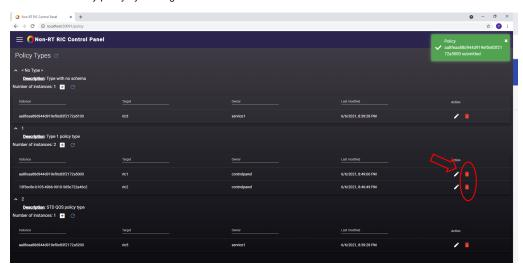
• Confirm deletion and verify the log on simulator side:
